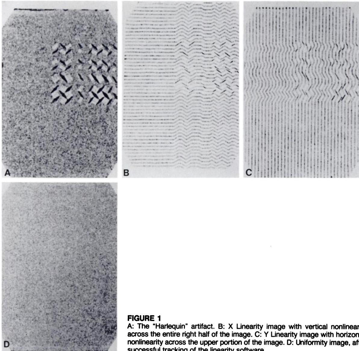
terns in the form of diamonds and squares—calls to mind the suit of clothes worn by a Harlequin, hence the appellation for the artifact. Acquisition of a flood image with all correction maps disabled resulted in the appearance of photomultiplier tubes (the consequence of no energy correction); otherwise, the image was unremarkable. Absence of the "Harlequin"
