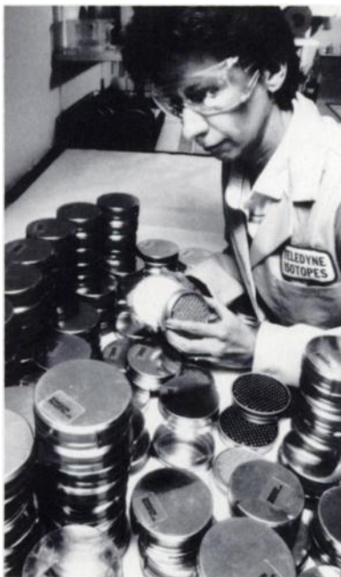
These activated charcoal canisters have been exposed for four days to the air inside various buildings being tested for radon levels. A scintillation detector can be used to measure the gamma radiation generated by radon daughter products. (Courtesy of Teledyne, Inc.)
