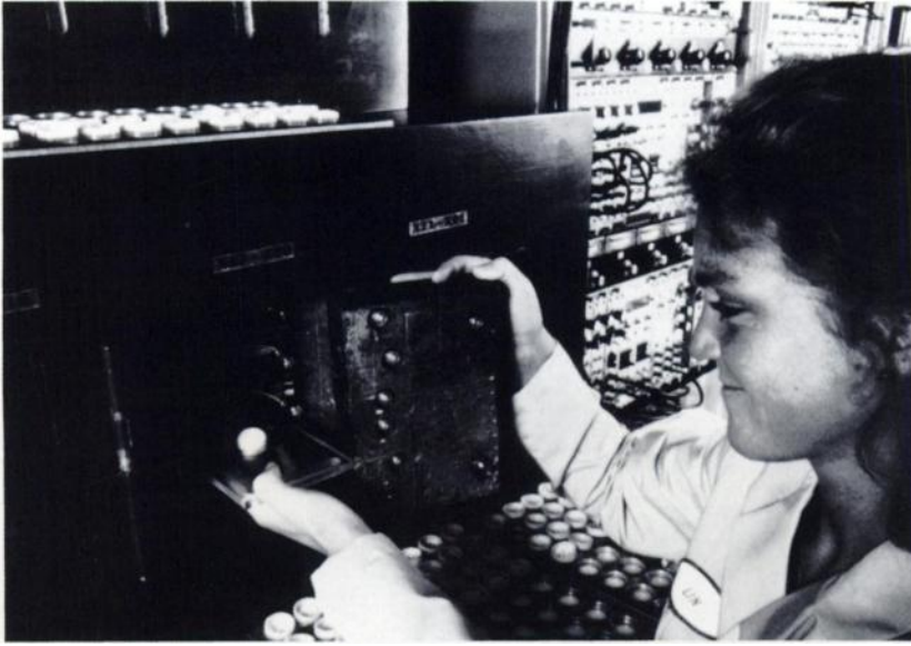
Soil samples from proposed building sites can be evaluated to determine radon concentrations by using a low-level beta detector (above) to measure the content of lead-210, a decay product of uranium.
