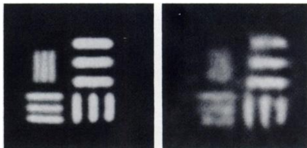
FIGURE 4 Resolution phantom. The image on the left is a planar image of the resolution phantom obtained by placing the phantom in contact with the collimator face. The image on the right is a SPECT of the same phantom. This phantom is made of lucite and has slots milled in it in which various quantities of radioactivity can be placed and measures 15 × 15 × 5.1 cm thick. The slots measure 6.5 × 1.6; 5.0 × 1.3; 6.0 × 1.0; and 6.0 × 0.7 cm, respectively.
