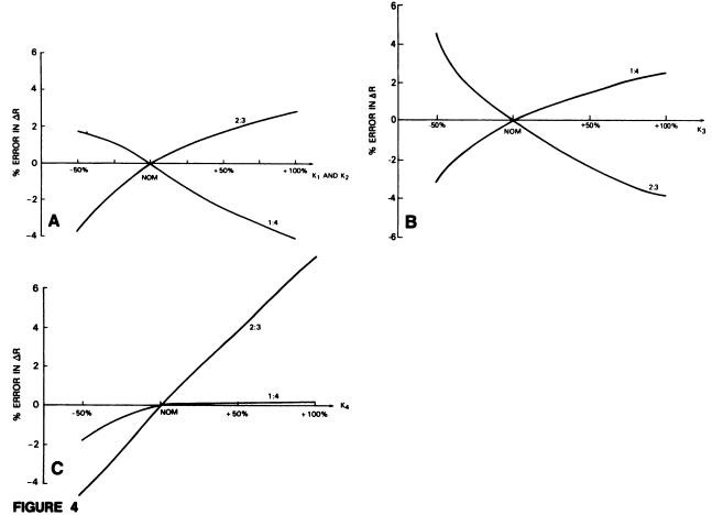
Net error in  $\Delta R = R_{RETEST} - R_{TEST}$  when the rate constants deviate from nominal in all terms, expressed as a percent of  $R_{TEST}$ . (A)  $k_1 - k_2$  deviation. (B)  $k_3$  deviation. (C)  $k_4$  deviation.
