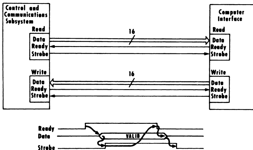
FIGURE 6 Communications protocol between RDAS Control and Communications Module and computer interface
