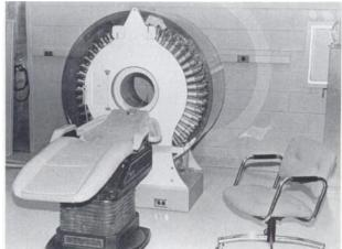
FIGURE 11 PETT V, first positron emission tomograph utilizing wobble motion of detectors to achieve suitable linear sampling
