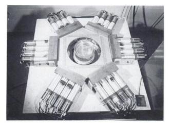
FIGURE 9 Early positron emission tomograph constructed from probes shown in Fig. 7
