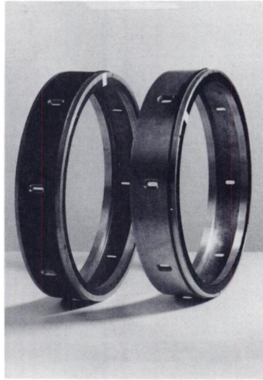
FIG. 2. High-resolution and high-efficiency aperture rings. Rings are gear-driven by microprocessor-controlled stepping motor. Optically sensed mark on rim of each ring is used to fix starting position.
