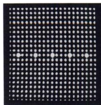
FIG. 9. Image of Smith orthogonal hole phantom obtained with Am-241 source at 1.5 m distance and detector event rate of 100,000 cps.
