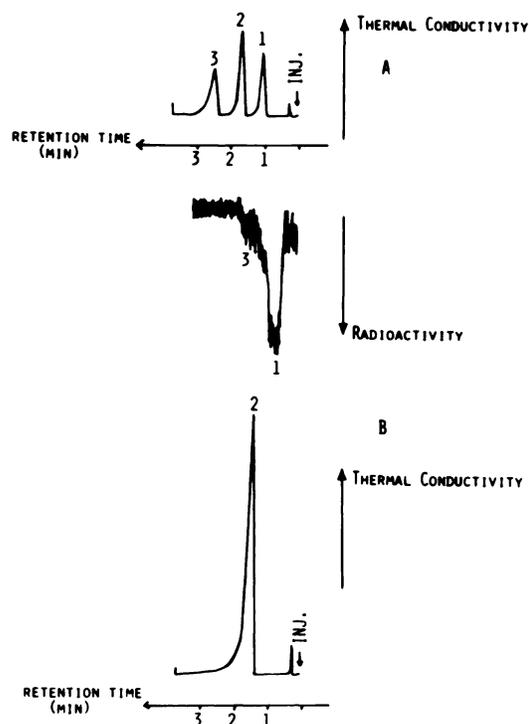
FIG. 4. Radiogaschromatography. Peak 1 = formaldehyde, Peak 2 = water, Peak 3 = methanol. A = test mixture; B = C-11 formaldehyde solution. Peak 1 represents 93.5% of the activity, Peak 3, 6.5%.
