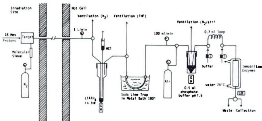
FIG. 2. Setup of C-11 formaldehyde production. ① = Pump 1. ② = Pump 2.
