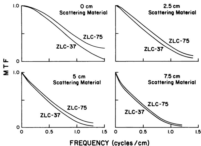
**FIG. 1.** Modulation transfer functions (MTFs) measured at various distances from collimator, using indicated camera, high-resolution, low-energy collimator, and 20% symmetric energy window. For all distances greater than 0 cm, region between collimator and source was occupied by tissue-equivalent scattering material. Note progressive diminution in difference in resolution between two cameras with progressive increase in distance from collimator.
