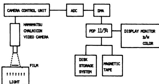
FIG. 1. Schematic diagram of TV-film analysis system. Video signals of light intensities transmitted through ARG films are digitized by ADC, transferred to PDP 11/34A through DMA interface, and archived in a magnetic-disk storage system.
