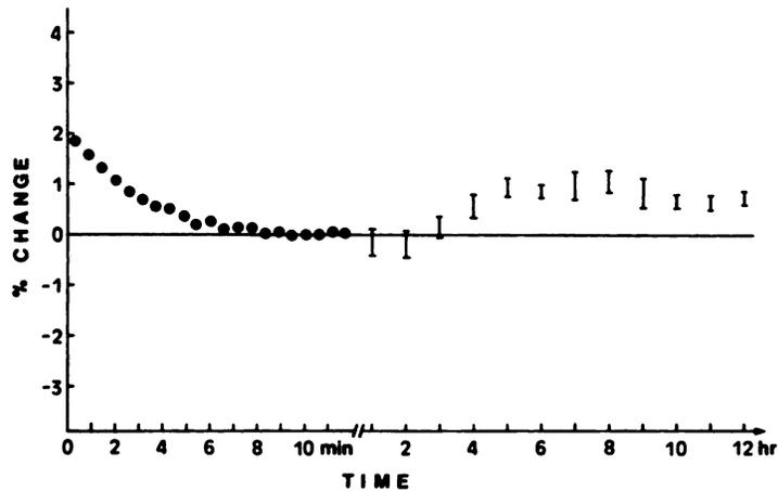
FIG. 5. Stability of system. Light intensity in center of field of view was digitized for 12 hr. Values are shown as percent change from that at 10 min after initially turning on the system. Maximum range within every hour is shown for first 12 hr.
