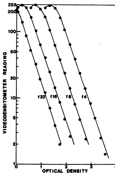
FIG. 4. Relation between optical density and digitized light intensity with different lens openings.
