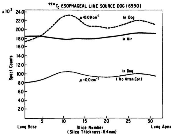
FIG. 4A, 4B. Line-source evaluations in dog esophagus and in air. SPECT counts obtained from ROI data are shown for each of 32 contiguous transaxial images. First and last slices correspond to lung base and apex. Value of  $\mu = 0.09/\text{cm}$  was used for attenuation coefficient with the first-order algorithm. Data indicated by  $\mu = 0.00/\text{cm}$  has not been compensated for attenuation. Note increased attenuation at lung base due to effects of heart and liver.
