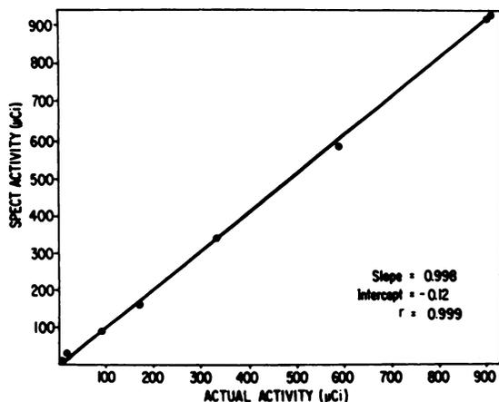
FIG. 2. Relationship between calculated SPECT-measured activity of point sources in air and actual activity ( $\mu\text{Ci}$ ).
