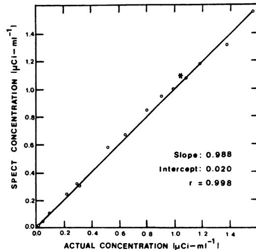
FIG. 1. Relationship between calculated SPECT concentration ( $\mu\text{Ci/ml}$ ) and actual concentration of distributed extended source in a cylinder 22 cm in diameter. A constant calibration factor was determined using the Tc-99m 1.08  $\mu\text{Ci/ml}$  source.
