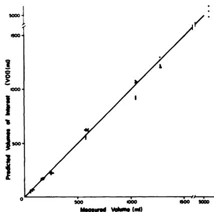
FIG. 1. Correlation of volumes of plastic cylinders containing  $^{99m}\text{TcO}_4^-$  in water, determined by computer program (macrofunction) using single-photon emission scintigraphic data compared with measured volume. At each volume, three points on ordinate are shown, representing three planes studied.
