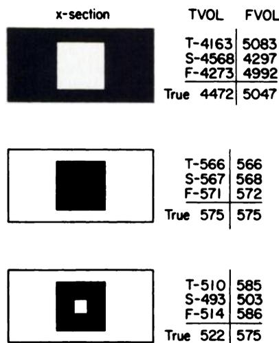
FIG. 2. Configuration of Lucite cylinder phantoms containing water (white) and  $^{99m}\text{TcO}_4^-$  dispersed in water (black). Two computer programs (macrofunctions), TVOL and FVOL, were used to estimate volumes. TVOL estimated radioactive component only, excluding "holes"; FVOL included holes as well.
