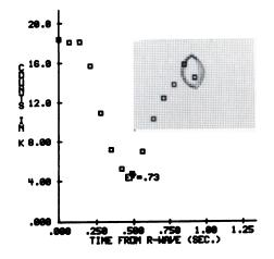
FIG. 4. Simulated gated pool acquisition at 60 cycles/min with framing rate of 0.07 sec/frame; acquisition time of 3 min; parallel-hole collimator. Count rate was ~4200/sec in systole. True EF = 75% (80 cc EDV and 20 cc ESV). Computer calculated EF = 73%.
