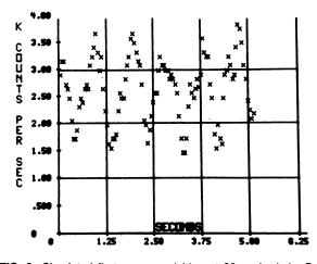
FIG. 3. Simulated first-pass acquisition at 60 cycles/min. Data points correspond to 0.1-sec intervals with 0.05-sec increments. Counts at end-systole points were as low as 146 (count rate of 1460/sec). True EF = 54%. Computer-calculated EF = 56%.
