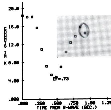
FIG. 4. Simulated gated pool acquisition at 60 cycles/min with framing rate of 0.07 sec/frame; acquisition time of 3 min; parallel-hole collimator. Count rate was ~4200/sec in systole. True EF = 75% (80 cc EDV and 20 cc ESV). Computer calculated EF = 73%.
