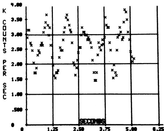
FIG. 3. Simulated first-pass acquisition at 60 cycles/min. Data points correspond to 0.1-sec intervals with 0.05-sec increments. Counts at end-systole points were as low as 146 (count rate of 1460/sec). True EF = 54%. Computer-calculated EF = 56%.
