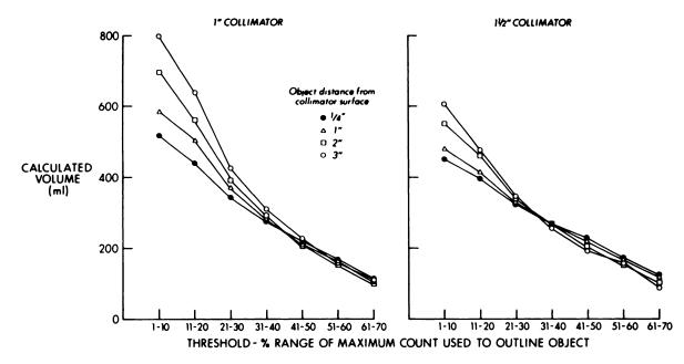
FIG. 2. Calculated volume of spherical phantom using different thresholds for the borders, expressed as a function of maximum counts in image, at different distances from collimator. 1.0-in. collimator (left); 1.5-in. collimator (right).
