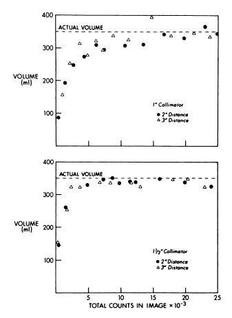
FIG. 1. Plot of estimated volume of spherical phantom as a function of total counts in image using either 1.0- or 1.5-in. collimator. Phantom's true volume was 350 ml.
