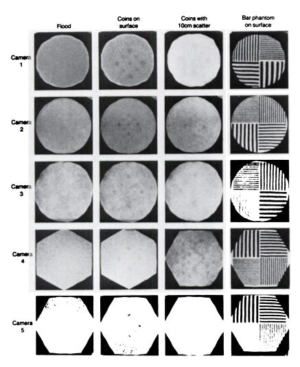
FIG. 2. Examples of daily quality assurance images from five gamma cameras. Columns present, left to right, two-millioncount flood source on collimator surface, two-million-count coin phantom image on collimator surface, two-million-count coin phantom image with 10 cm of Plexiglas, and two-million-count bar phantom on collimator surface. Rows represent data for Cameras 1–5 as listed in text.
