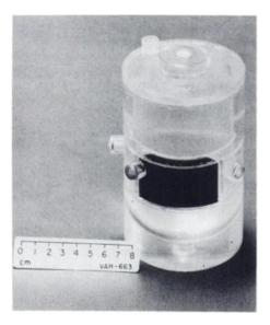
FIG. 1. Photograph of heart phantom; whose design follows that of Mueller et al. (University of Iowa). The 24-cc chamber used as a perfusion defect has been identified with colored dye.
