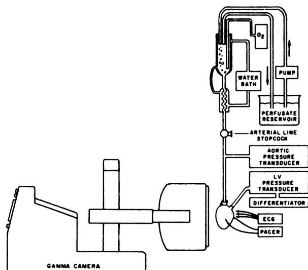
FIG. 1. Apparatus for the perfusion of isolated rabbit heart, with gamma scintillation camera in position for imaging.
