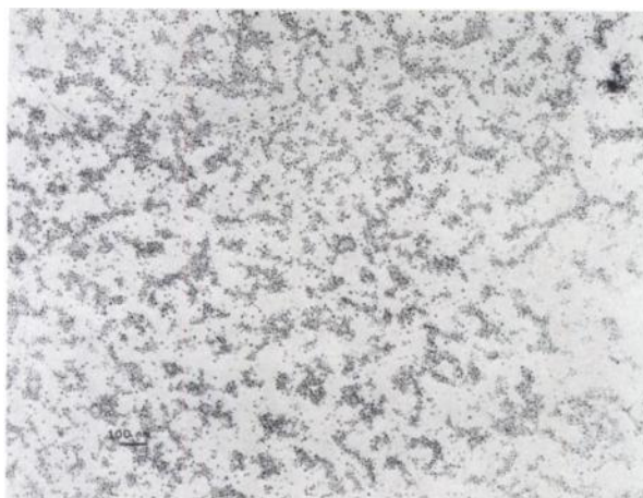
FIG. 2. Transmission electron micrograph of Tc-99m antimony sulfide colloid. Note fairly uniform particle size. Since the stabilizer, polyvinyl pyrrolidone, has a molecular weight of 10,000, it would be smaller than particles observed here and thus the micrograph shows the colloid that is formed.
