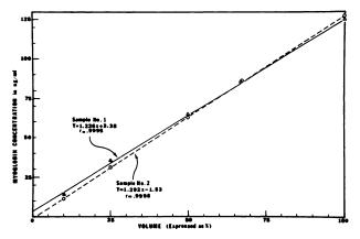
FIG. 2. Proportional dilution of two myoglobin samples confirms excellent test linearity. Ordinate shows measured myoglobin concentration; abscissa gives reciprocal of dilution factor, as percentage of original.
