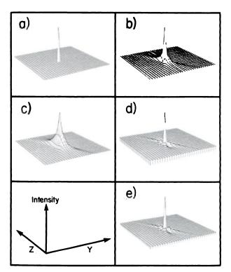
**FIG. 1.** Perspective drawings illustrating correction technique for out-of-focal-plane blurring. (A) Location of a point source in cross-sectional plane. (B) Point-source response function  $F(\tilde{r} - \tilde{r}')$  for source in (a). (C)  $F(\tilde{r} - \tilde{r}')$  after smoothing in y and x directions. (D)  $DS F(\tilde{r} - \tilde{r}')$ . (E)  $E F(\tilde{r} - \tilde{r}')$ .
