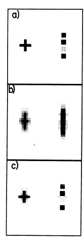
FIG. 2. Examples of simulated axial images before and after correction for out-of-focal-plane blurring. (A) Location of sources in cross-sectional plane. Source distribution on left is three-dimensional cross of activity with arms of equal length in y, z, and, hidden in this view, x directions. (B) Distorted images reconstructed using back projection. (C) Images corrected for out-of-focal-plane blurring.
