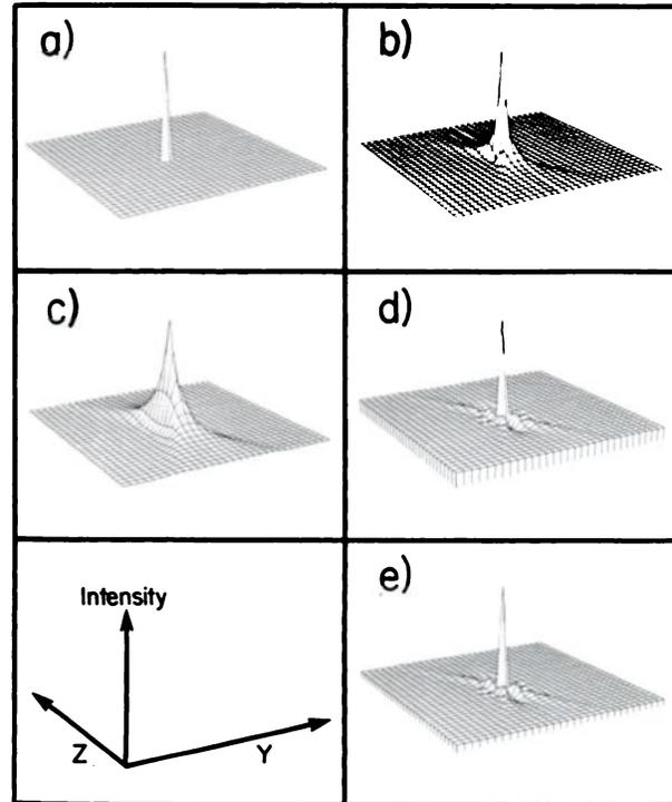
FIG. 1. Perspective drawings illustrating correction technique for out-of-focal-plane blurring. (A) Location of a point source in cross-sectional plane. (B) Point-source response function  $F(\vec{r} - \vec{r}')$  for source in (a). (C)  $F(\vec{r} - \vec{r}')$  after smoothing in  $y$  and  $x$  directions. (D)  $DS F(\vec{r} - \vec{r}')$ . (E)  $E F(\vec{r} - \vec{r}')$ .
