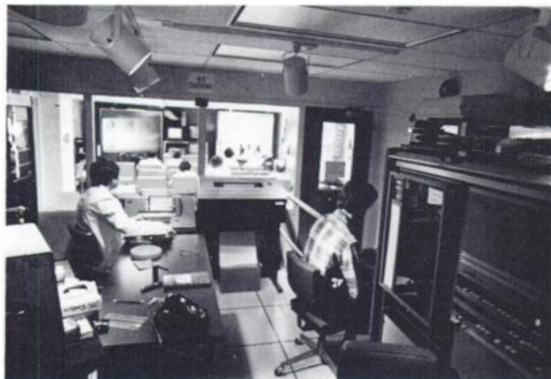
FIG. 2. Consultation room is viewed from data processing room. Glass walls permit good visual communication and prevent computer noise from reaching other areas.
