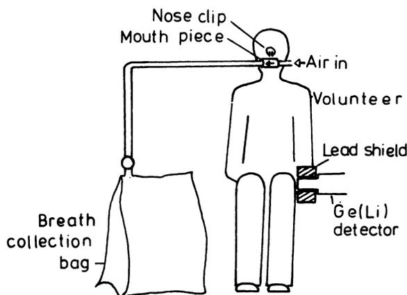
FIG. 1. "Open circuit" breath-collection system. The Ge(Li) detector monitoring activity in subject's thigh is also shown.
