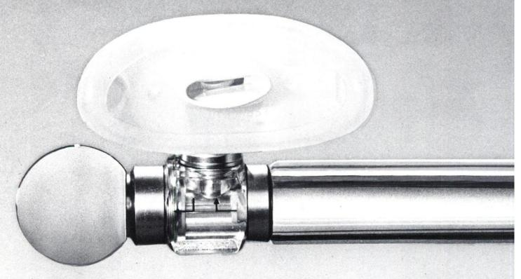
Everybody benefits from comprehensive technological advances like the widely used Omnimedical AVM-3 Automated Ventilation Module. With the AVM-3 radioxenon ventilation studies are automated, simplified, reproducible one man operations. Patient cooperation is not needed. Interfaced with the gamma camera, the operator selects a study sequence-Single Breath (tidal volume or vital capacity) or Rebreathe, singly or in combination - and pushes the start
