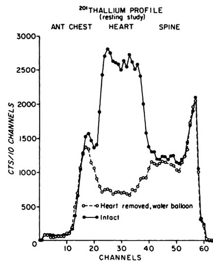
**FIG. 5.** Direct comparison of horizontal profiles with heart intact and with heart replaced with water balloon. Activity surrounding heart greatly exceeds true background activity. Effect of scatter from heart into surrounding region can be appreciated.
