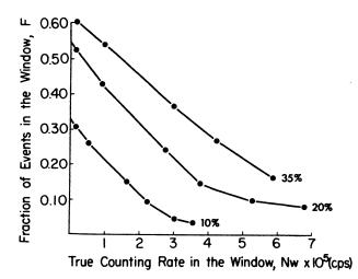
FIG. 3. Fraction of events in window plotted as function of true event rate in that window. Curves for Tc-99m in 10%, 20%, and 35% windows.
