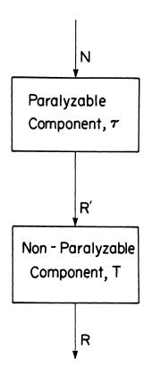
FIG. 1. Paralyzable—nonparalyzable counting system. Output of paralyzable component is input to nonparalyzable component.
