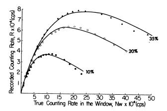
FIG. 4. Observed vs true event rates for Pho/Gamma IV camera at  $\bullet$  10%,  $\bigcirc$  20%, and  $\triangle$  35% window widths. Solid lines are data obtained from decaying-source method. Points are calculated from Eq. 5 using parameters in Table 1.
