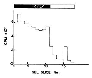
FIG. 3. Separation of proteins in streptase by polyacrylamidegel electrophoresis. Procedure as described in section on methods and materials. Top part of diagram shows diagrammatic representation of gel as stained for protein. Lower part shows distribution of <sup>90m</sup>Tc in different sections of gel.
