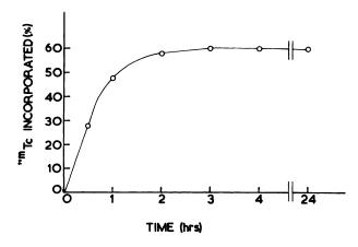
FIG. 1. Time course of <sup>99m</sup>Tc incorporation into streptokinase. Reaction mixture contained streptokinase 50,000 I.U., stannous pyrophosphate 1 mM, and <sup>99m</sup>Tc. Values are means of three separate experiments each carried out in duplicate.
