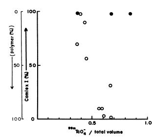
FIG. 3. Effect of <sup>99m</sup>TcO<sub>4</sub><sup>-</sup> concentration on Complex I formation. Concentration of <sup>99m</sup>TcO<sub>4</sub><sup>-</sup> is expressed as ratio of added <sup>99m</sup>TcO<sub>4</sub><sup>-</sup> volume to total volume of labeling solution. Efficiency was determined by Sephadex column chromatography.
