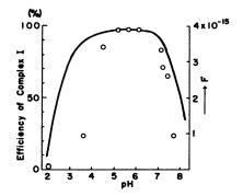
FIG. 2. Effect of pH on Complex I formation. Circles represent labeling efficiencies determined by Sephadex column chromatography. [Labeling conditions:  $4 \times 10^{-5}$  M SnCl<sub>2</sub> (0.5 ml) was added to mixture of  $10^{-2}$  M Pen (1.5 ml) and <sup>sem</sup>TCO<sub>4</sub><sup>-</sup> (3 ml); pH was adjusted with acetate buffer or HCl (3 ml).] Curve corresponds to calculated F-value (Ko<sub>H</sub>[H<sup>+</sup>]<sup>2</sup>[PEN]<sup>3</sup>).
