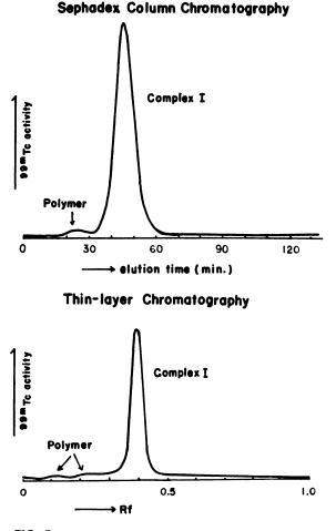
FIG. 5. Typical results of Complex I on Sephadex column chromatography and thin-layer chromatography. Sephadex column chromatography: Sephadex G-15, 2.0  $\times$  17-cm column, 0.15 M NaCl elution solvent, 108 ml/hr flow rate. Thin-layer chromatography: Toyo Kasei silica gel spot film, n-butanol-acetic acid-water, 4:1:1.
