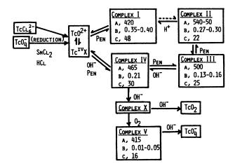
FIG. 1. Labeling products of <sup>som</sup>Tc-Pen reaction. (A) Wavelength of absorption maximum (nm). (B)  $R_r$  value on thin-layer chromatography (n-butanol-acetic acid-water, 4:1:1). (C) Elution time (min) in Sephadex G-15 column chromatography (flow rate = 108 ml/hr).
