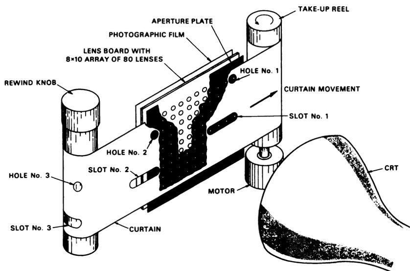
**FIG. 1.** Schematic drawing of first 80-lens camera. Holes are aligned with beginnings of respective slots as described in text. (Drawing assumes cathode-ray tube image to be upside-down.)
