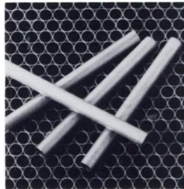
FIG. 2. Section of Ta collimator with superimposed individual tantalum tubes.
