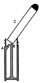
FIG. 1. Cross section of liquid scintillation vial with (A) lateral protuberance, (B) central stem, and (C) RIA tube.
