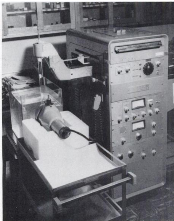
FIG. 1. Automated method for scanning of efficiency distribution of single-bore, nonfocused collimators. Probe combined with collimator separated from scanner is held in fixed position. Probe is electronically connected to scanner display. Point source of radionuclide attached to scanner arm is moved through water phantom in collimator field of view.
