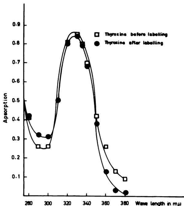
FIG. 4. Ultraviolet spectra of  $T_4$  before and after labeling.
