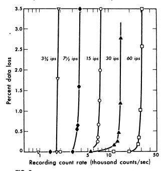
FIG. 3. Percent data loss is shown as function of input counting rate from scintillation camera for each recording speed. Data loss remains insignificant until near saturation when recorded counting rate rapidly approaches maximum value for each recording speed.
