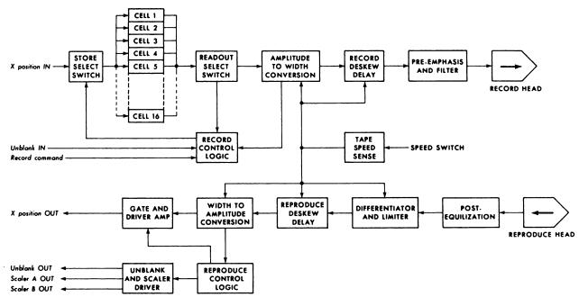
FIG. 1. Block diagram of analog recorder system. Signalprocessing functions are shown only for x coordinate channel. y co-
