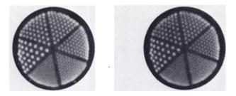
FIG. 4. Test patterns: (left) Original data from scintillation camera; (right) recorded first and photographed on playback. No distortion or loss of spatial resolution can be seen.
