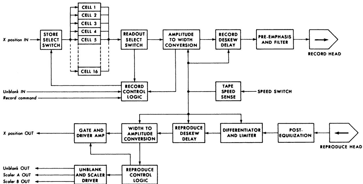
**FIG. 1.** Block diagram of analog recorder system. Signal-processing functions are shown only for x coordinate channel. y co-
