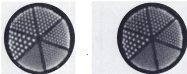
**FIG. 4.** Test patterns: (left) Original data from scintillation camera; (right) recorded first and photographed on playback. No distortion or loss of spatial resolution can be seen.
