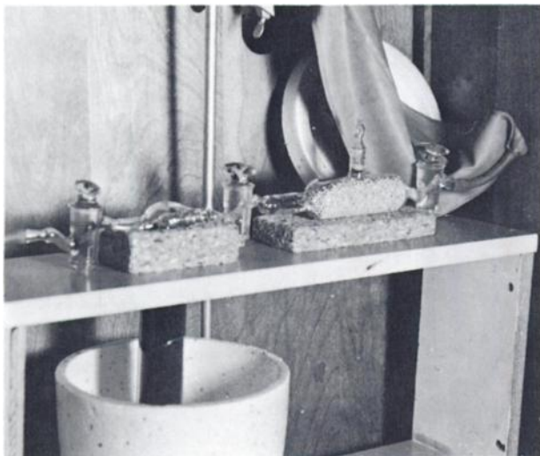
FIG. 2. First trap with moisture pretrap arranged for cooling.
