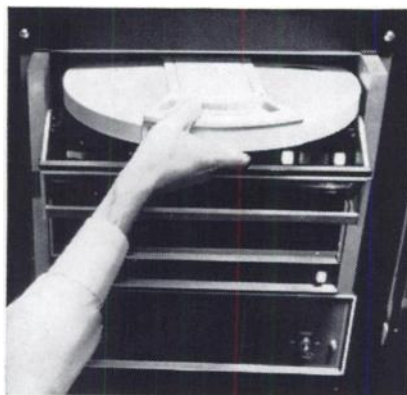
The disk retrieves stored information in milliseconds. To get any result from the disk quickly, simply tap two letters on the teletype keyboard.
