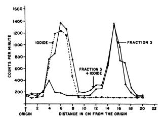
FIG. 4. Paper chromatographic separation of third fraction and iodide in butanol, acetic acid, and water (78:5:17) system for 18 hr. One-centimeter strips were cut and counted in well scintillation counter.
