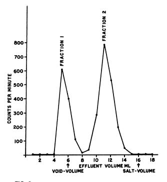
**FIG. 1.** Typical pattern of separation of damaged and free radioinsulin on sephadex G-75. Stock <sup>125</sup>I-insulin (0.1 ml) was incubated with 0.05 ml of iodoacetamide treated plasma at  $37^{\circ}$ C for 30 min and passed on sephadex G-75 column (1  $\times$  12 cm). Column was eluted with 0.025 M phosphate buffer containing bovine serum albumin.
