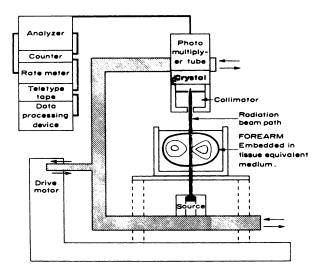
FIG. 1. Principle of Cameron-Sorenson bone mass determination. Photon beam is moved across limb at 4.5 cm/min; count is printed every 1.5 sec. Data can be processed by planimetry or computed electronically. Amount of bone mineral in path of beam is related to transmission counting rates. (From Riggs BL, Jowsey J, Kelly PJ, Wahner HW: Special procedures for assessing metabolic bone disease. M Clin North Am 54: 1061–1070, 1970. By permission of WB Saunders Co.)
