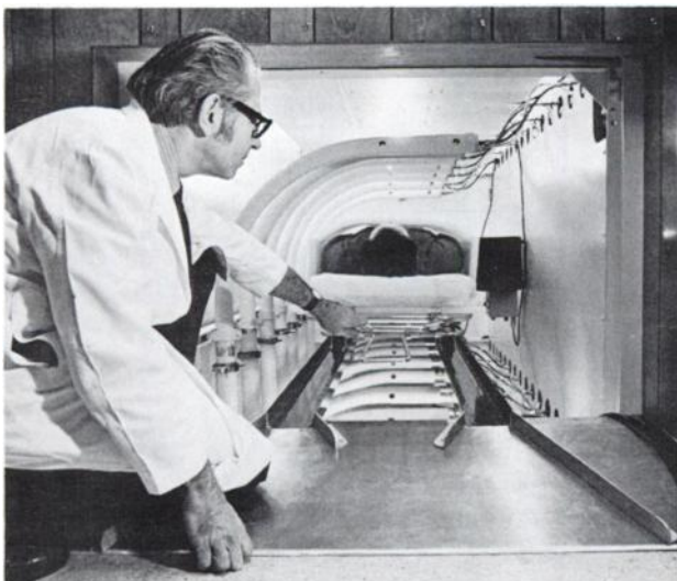
FIG. 1. ^{238}\text{Pu,Be} neutron irradiation facility. Patient is positioned as shown between upper and lower guide tubes which are used to position fourteen 50-Ci sources of ^{238}\text{Pu,Be} .
