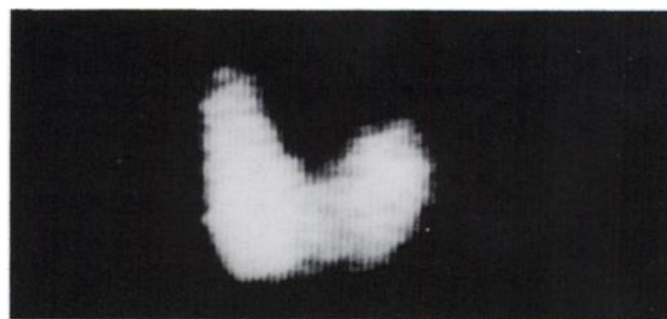
FIG. 3. Reconstructed image of 10- \mu Ci thyroid phantom taken with lead zone plate (on-axis) and Anger camera.
