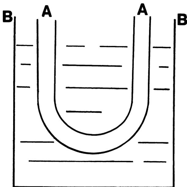
**FIG. 1.** Schematic apparatus for dialysis method. (B.B. = receptor vessel with normal saline. A.A. = loop of dialysis tubing for labeled sample.)
