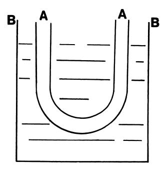
FIG. 1. Schematic apparatus for dialysis method. (B.B. = receptor vessel with normal saline, A.A. = loop of dialysis tubing for labeled sample.)
