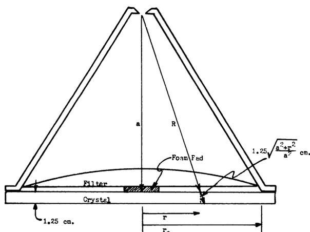
FIG. 1. Geometry of pinhole collimator and correction filter.
