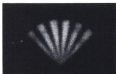
2. Pho/Gamma-HP 50,000 counts, 70 seconds 2 inches from High Resolution Collimator
