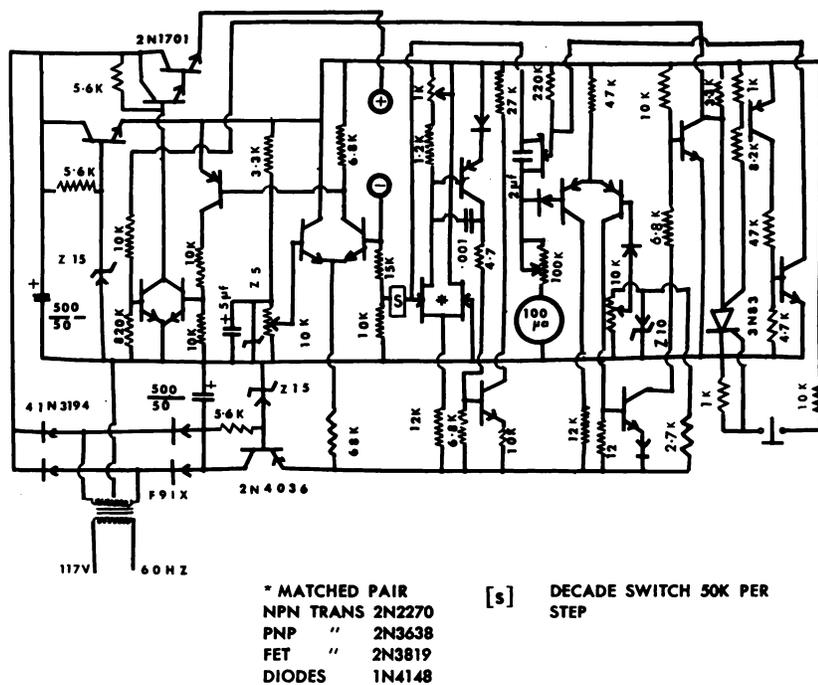
FIG. 1. Circuit diagram of constant charge generator.
