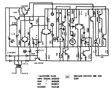
FIG. 1. Circuit diagram of constant
