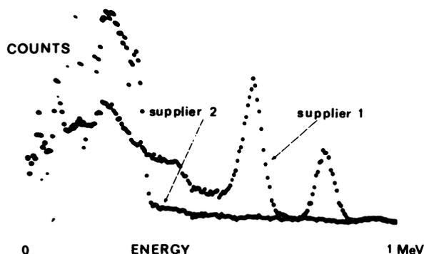
FIG. 3. Comparison of spectral characteristics of eluants from generators of Suppliers I and II.
