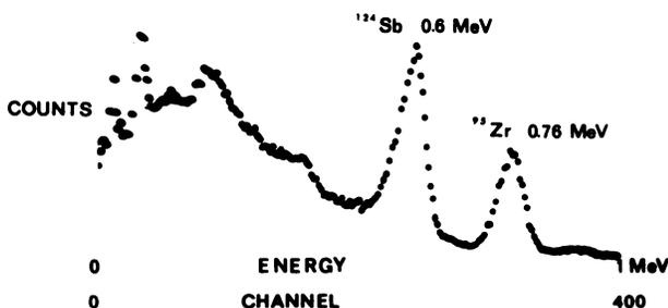
**FIG. 1.** Spectrum of activity seen in eluates from generators of Supplier I 3 days after elution showing contaminants.
