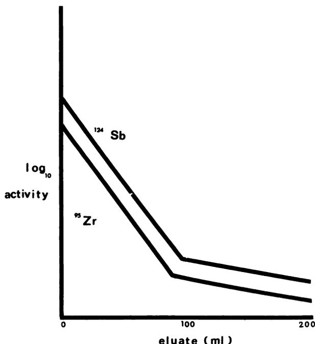
FIG. 2. Zirconium-95 and  $^{124}\text{Sb}$  levels after repeated elutions of generator.
